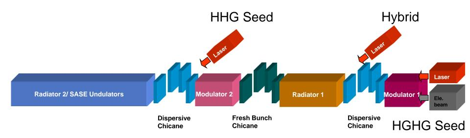
Structure given by cascaded HGHG HHG seed at entrance of SASE undulators=radiator 2 HHG seed at entrance of radiator 1 combined with 1 HGHG stage
