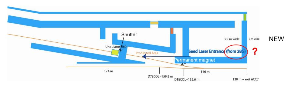
In both cases (old/new) HHG seed details are unclear (but will be in one of the HGHG chicanes) Safety issues need to be clarified, but shutter and space for "permanent" magnet needed
