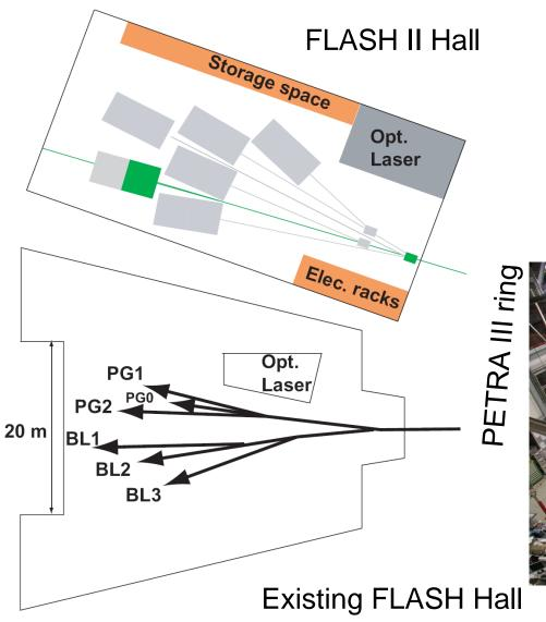
More space for experiments Two experiments in a row Less mirrors to experiment
