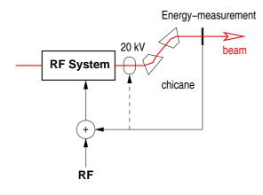
Although there are particular setpoints where the RF stability is not critical, a **beam based feedback** looks necessary in any case, not to be limited.
