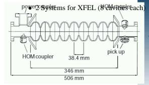
TESLA type cavities have been scaled down in size to fit the 3.9 GHz. All auxiliaries like coupler, HOM coupler, frequency tuner, etc..., are scaled as well. Most of this work was done by H.Edwards et al. / FNAL. 3
