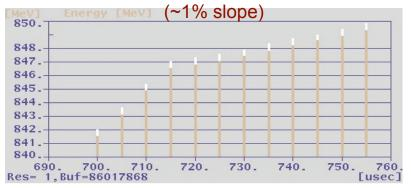
Energy slope along the bunch-train shows second-order dispersion on the orbits of the individual bunches
