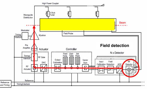
Drifts from Field Detector are amplified and pushed onto the beam.
