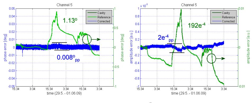
Compensation of phase drift : ~ 1/140 Compensation of amplitude drift : ~ 1/100
