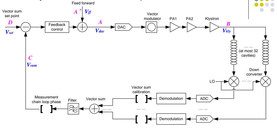
→ Taking into account the feedback (here is a P controller), the closed loop gray box model is
