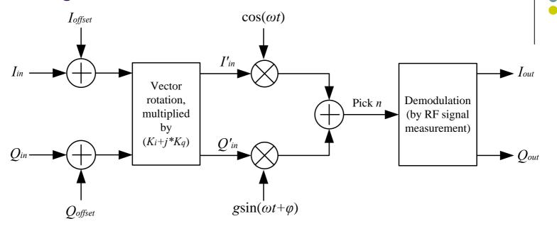
Unknown parameters:  $I_{offset}$ ,  $Q_{offset}$ ,  $K_i + jK_q$ , g,  $\varphi$
