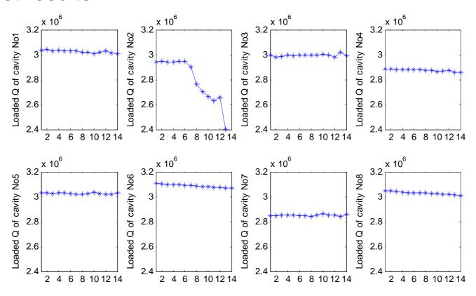
Loaded Q measurement at the RF decay part for each cavity of ACC1, the x number means 14 times measurement with different set point gradient (from 9.3MV/m to 10.6MV/m, 0.1MV/m as increment steps)
