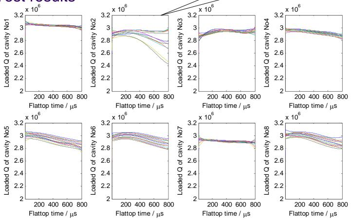
Loaded Q measurement during RF flattop for each cavity of ACC1, the curves for each cavity means 14 times measurement with different set point gradient (from 9.3MV/m to 10.6MV/m, 0.1MV/m as increment steps)
