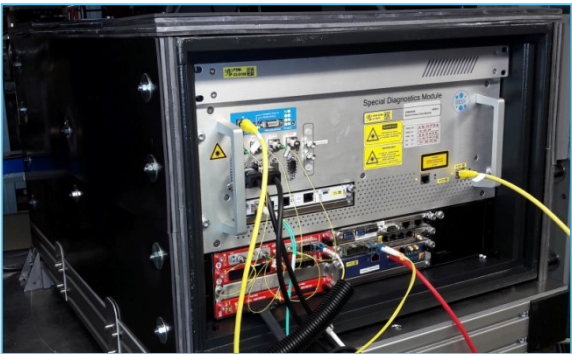
“BAM-box” with EO modulator MTCA.4 crate (2HE) with ADCs.
