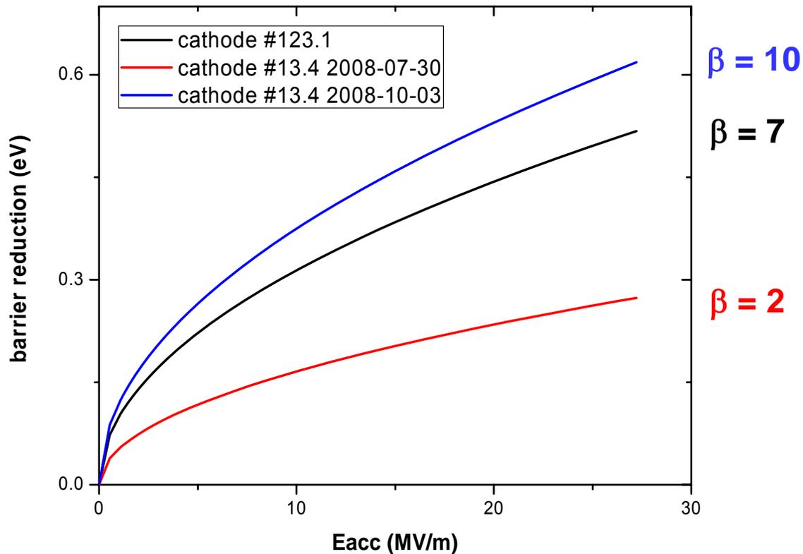
The theoretical electron affinity of the cathodes is 0.2 eV. The obtained lowering of the work function is higher than expected, but the uncertainty of this parameter is rather high.
