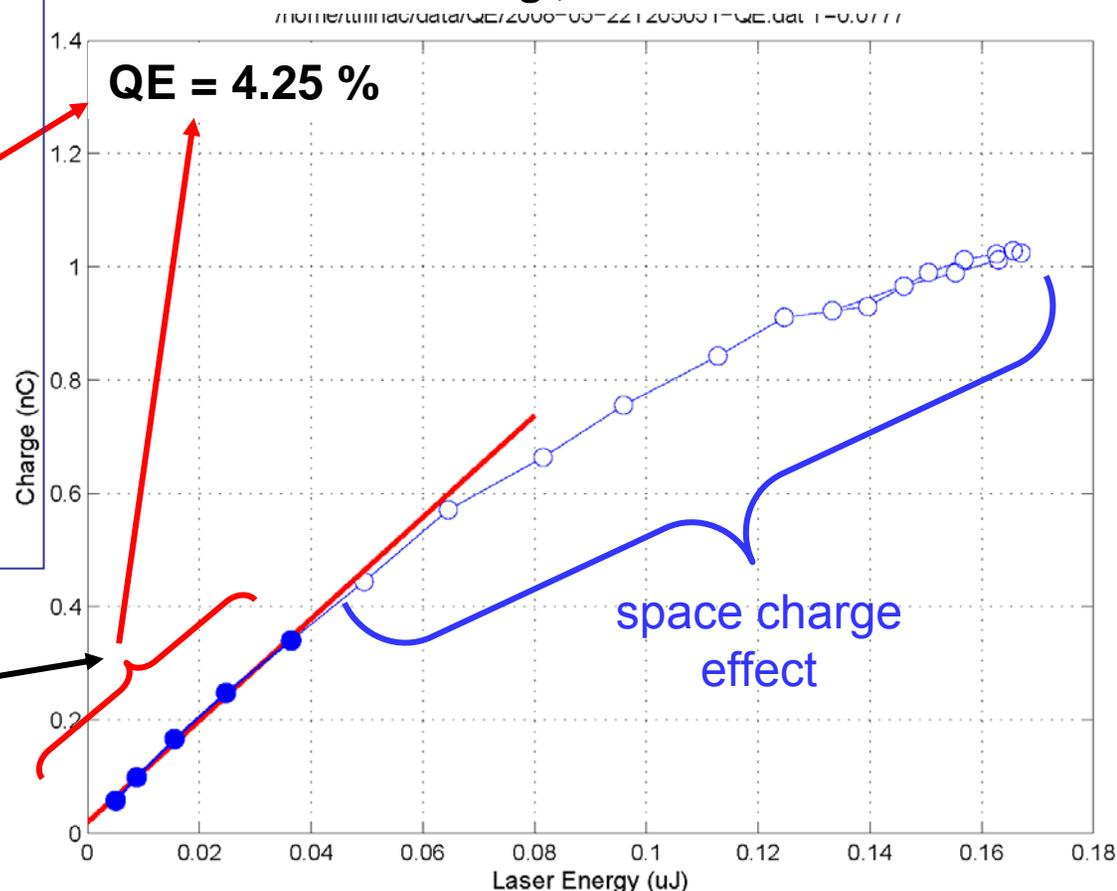
Charge versus laser energy obtained for different laser diameters at the cathode, accelerating field constant.
