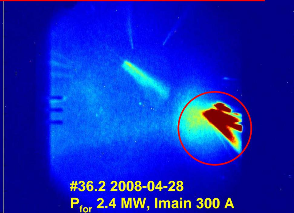
On this cathode lots of dust particles could be found. The reason was accidentally missing  $N_2$  flushing of the cathode before insertion into the box.
