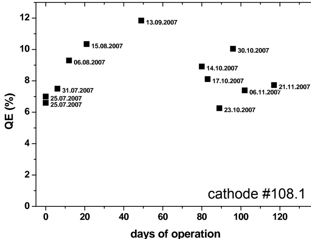
Since shut down works 2007 in the gun region (improved vacuum, removed teflon washers) an increased lifetime is observed.
