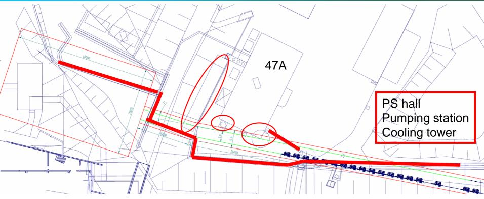
Cables/pipes along FLASH, crossing 47A, (new) cables at position experimental hall, He pipes etc. from 47A towards tunnel (FLASH backup)
