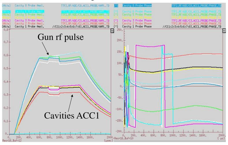
• in this case the Reflected power cable from gun was damaged
