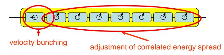
Velocity bunching is an additional "knob" to optimise the bunch compression system.
