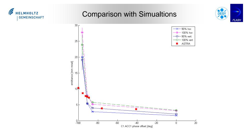
Measured emittance at phase offsets around -90 to -100 degrees disagrees with the simnualtions – possible reasons:
