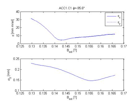
At full compression emittance after solenoid optimisation is 4.5mm mrad after ACC1.
