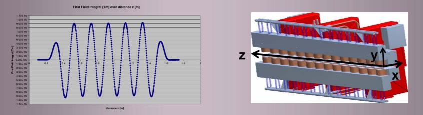
• At 0.3T of the radiator undulator which is be vertically placed gives values of  $-1.12 \times 10^{-5}$  Tm for the first field integral (  $<5 \times 10^{-5}$  Tm)
