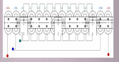
• For each undulator the field measurements were performed along the beam centerline (z-direction) for five different levels of peak field strength: 0.1, 0.2, 0.3, 0.4, 0.48T. The measurements at 0.3T were performed also at  $x = \pm 10$ mm and y = -4mm.
