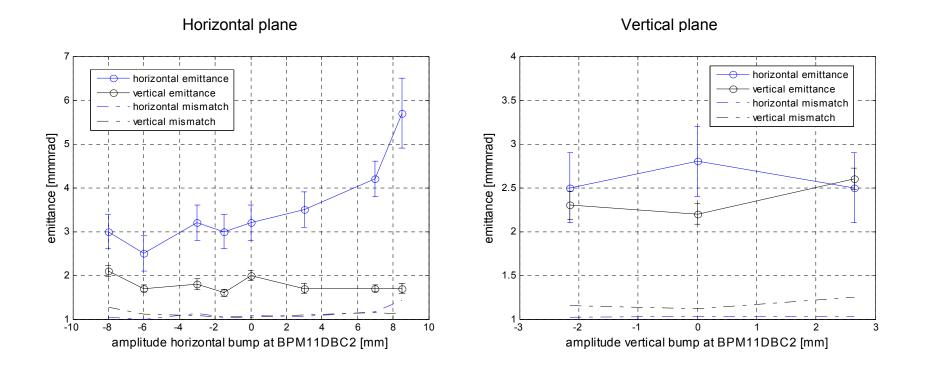
Horizontal plane: emittance increase only for positive bumps (maybe because the zero of this BPM is shifted)
