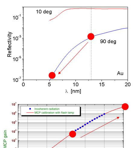
• MCP-2004 demonstrated good performance for SASE characterization and reliable detection of SASE radiation on top of background with winimum wavelength about 13 nm.
