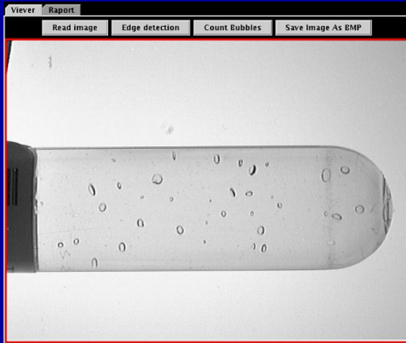
(a) Input: Digital photograph of the bubble dosimeter after neutron exposure
