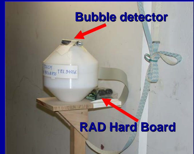
The Moderator, close up view (Bubble detector for in-situ calibration)
