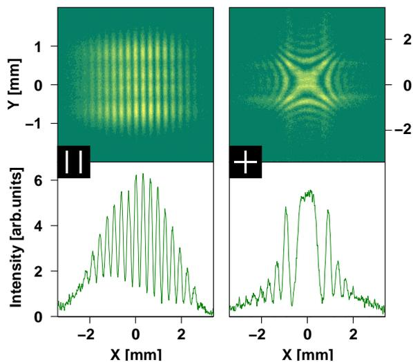
FIG. 10: Diffraction patterns of two different slit arrangements (see pictographs) illustrating the transverse coherence of the FEL radiation.
