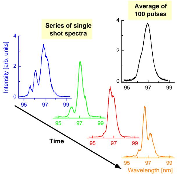
FIG. 6: Measured spectral distribution of the FEL radiation. Each single shot spectrum (originating from individual electron bunches) exhibits an ensemble of a few peaks corresponding to the fluctuation of the number of longitudinal modes of FEL radiation. This feature is characteristic for SASE FELs driven by shot noise. Since the center frequencies of these spikes are random (within the bandwidth of the FEL), they are smeared out in the averaged spectrum shown in the upper right corner.
