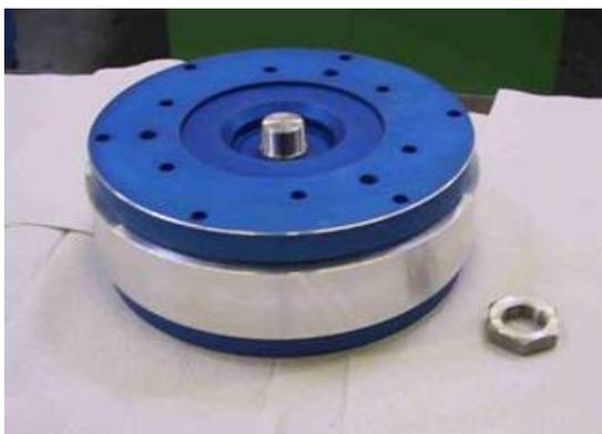
**Figure 6: Assembled turning fixture**
