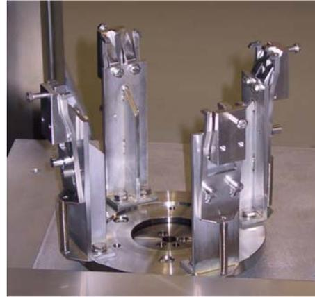
Figure 11: Iris tack- and welding fixture for the inside welding position
