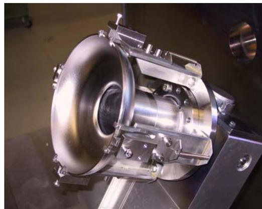
Figure 12: Welding fixture with installed half-cell and beam tube at  $45^\circ$
