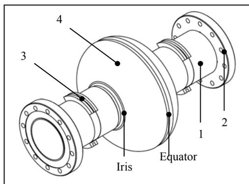
**Figure 1: Cavity with position number**
