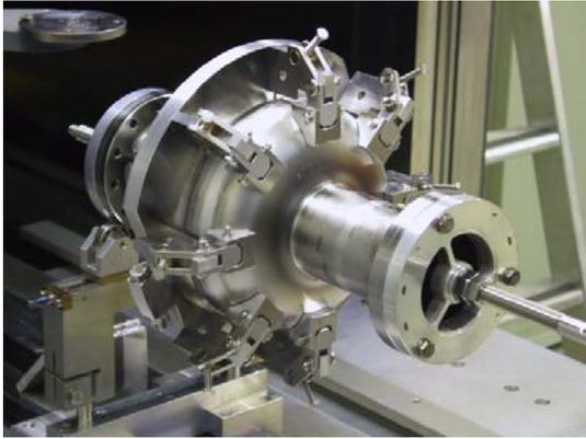
Figure 13: Tack weld fixture for equator
