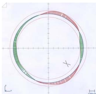
Figure 7: Example of a graphic display of large grain niobium's circularity
