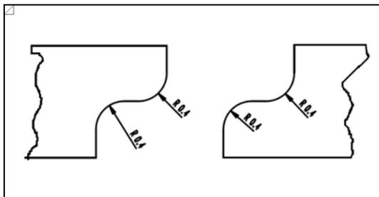
**Figure 3: Contour at the equator welding joint**
