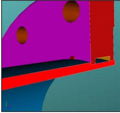
**Figure 2: Beam tube with leak search notch and -drilling**
