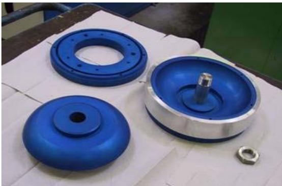
**Figure 5: Turning fixture for end half-cells**
