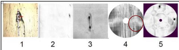
**Figure 4: Various inhomogeneities in niobium sheets**
