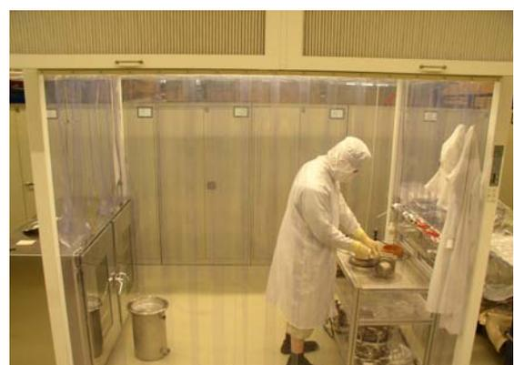
Figure 10: Local clean room with mounting area, vacuum transport container and N2 storing cabinet
