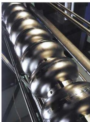
**Fig. 1: 1.3GHz nine cell Cavity**
