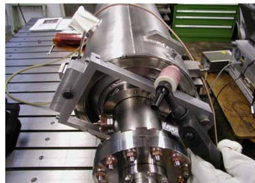
**Fig. 14: Tacking bellow side / Joint 3**
