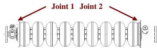
Fig. 8: Weld sequences at electron beam welding
