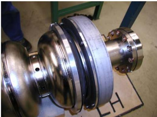
Fig. 7: Cavity long beam pipe side with bellow, fixture and shield on place
