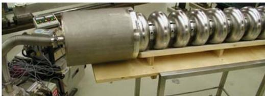
**Fig.10: Cavity with leak check container**
