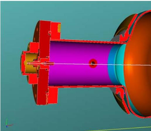
**Fig.5: FMS on long cavity side with Teflon tube clamping**
