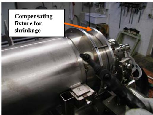
**Fig. 15: Tacking and adjusting sliding collar / Joint 4**
