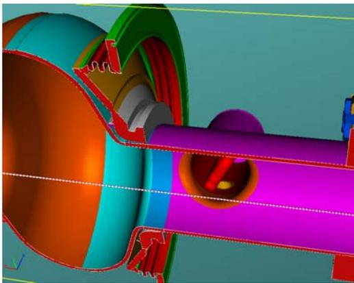
Fig. 6: Cavity long beam tube side with bellow
