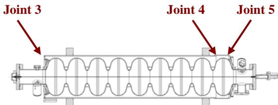
Fig. 11: Weld sequences at TIG welding the Helium vessel
