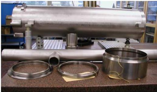
**Fig. 2: Helium vessel and parts**
