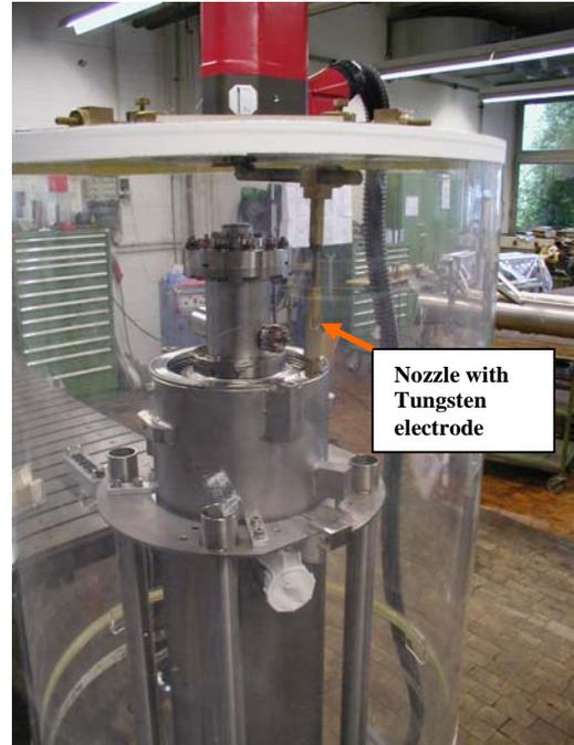
**Fig. 12: Cavity installed in a welding cabin rinsed with argon**
