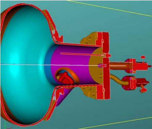
**Fig. 4: FMS on short cavity side with two valves, RF antenna and Teflon tube**
