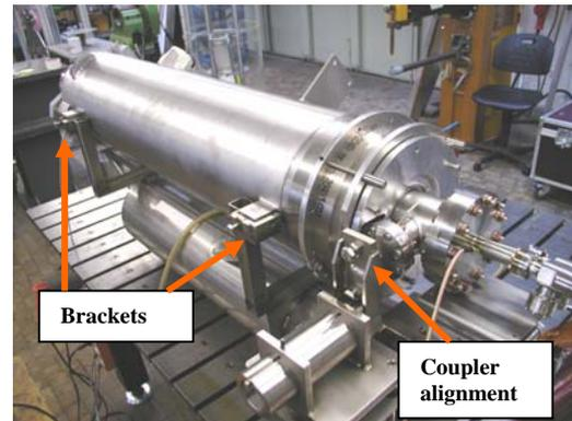
**Fig.13: Alignment Fixture for cavity to vessel**
