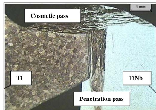
Fig. 9: Polished micro cut of Titanium-Niobium to Titanium electron beam weld
