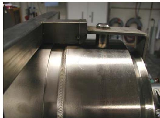
**Fig. 16: Adapter on sliding collar**
