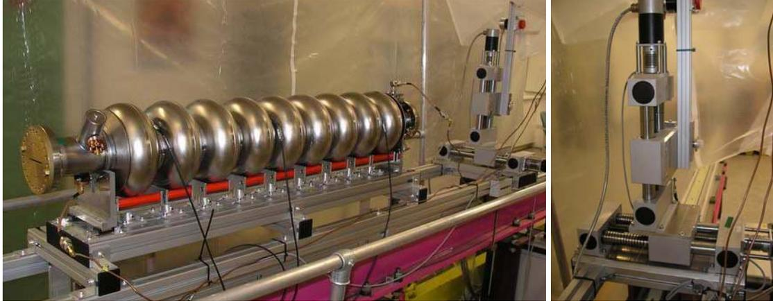
*Fig. 3.2 Cavity on the measurement setup (left) and detail of transmissions for transversal bead movement (right)*
