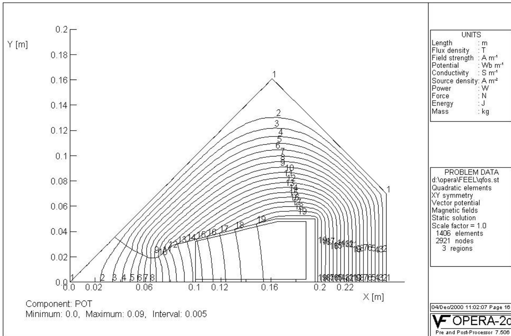
**Fig. II. 9 QFOC1. The map of the lines  $A=\text{const}$  , [T·m]**
