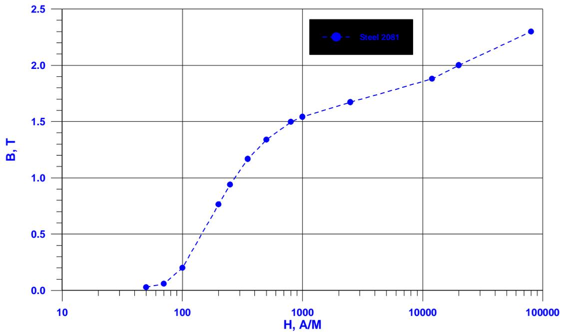
Fig. II. 1 The magnetization curve of the magnet steel.
