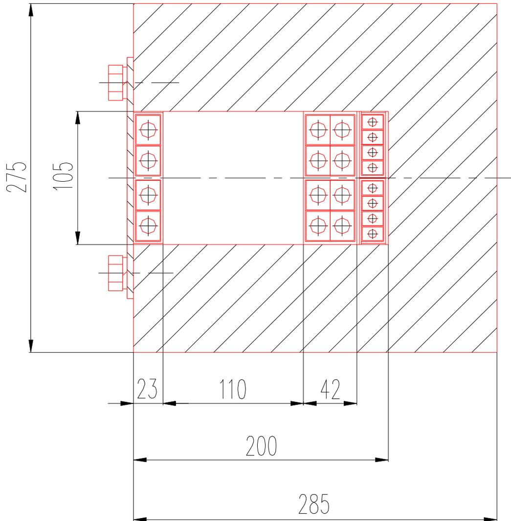
**Fig. II. 7 The cross section of SEPTUMT magnet**
