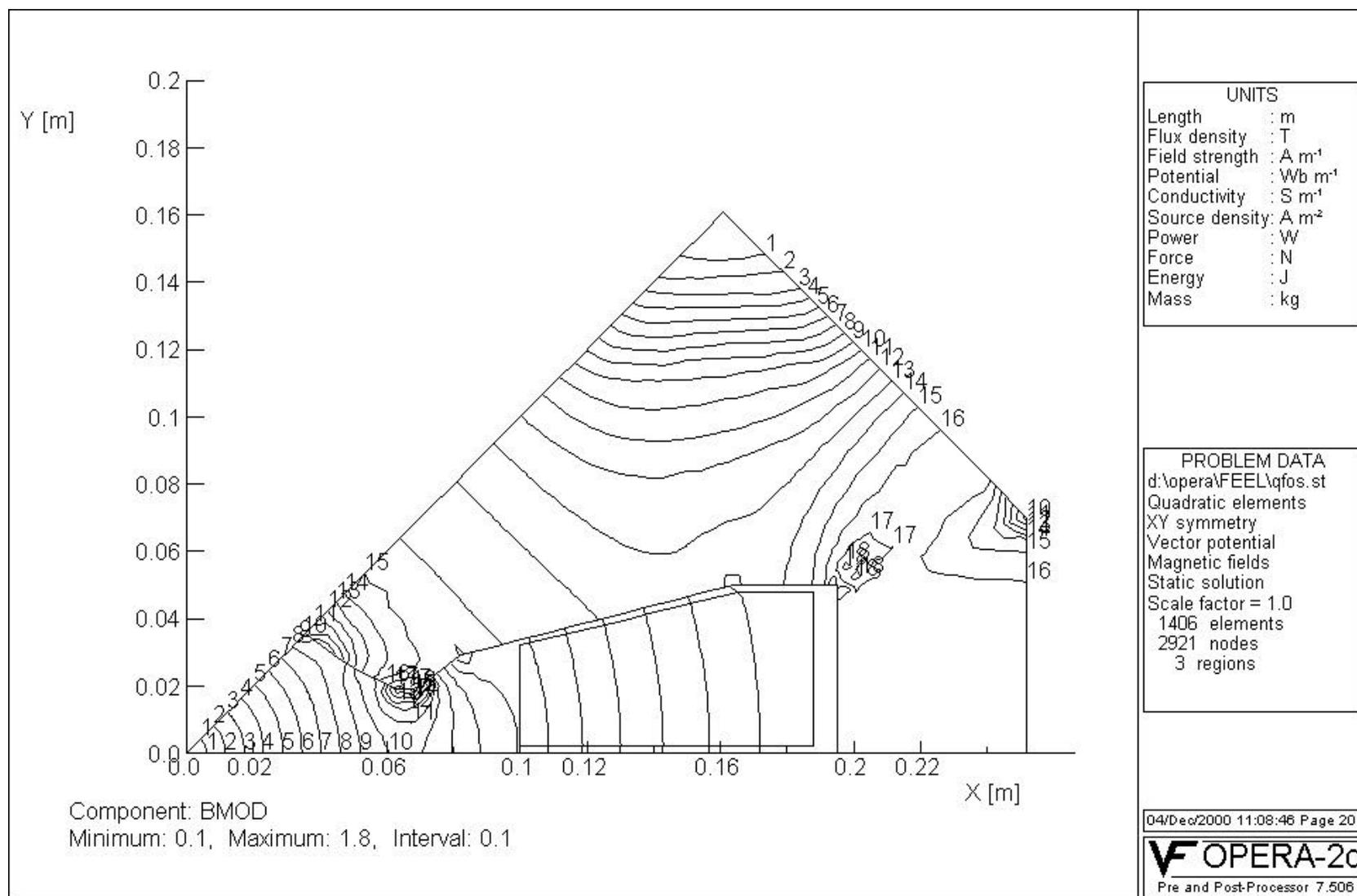
**Fig. II. 10 QFOC1. The map of the lines  $\frac{1}{2}B^2 = \text{const}$ , [T]
