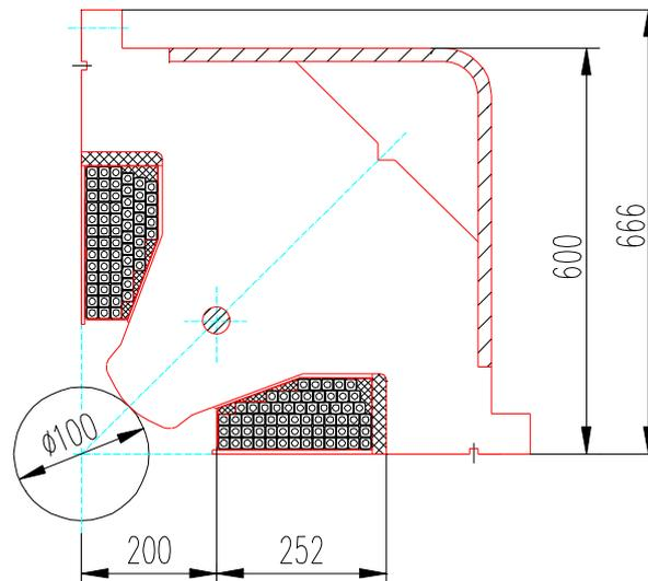
**Fig. II. 8** The cross section of the QFOC1, QDFOC, QFOC quadrupoles
