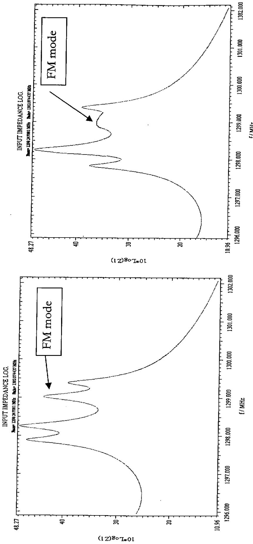
Transmission signal from the HOM coupler before suppressing of FM mode (2<sup>nd</sup> from the right).
