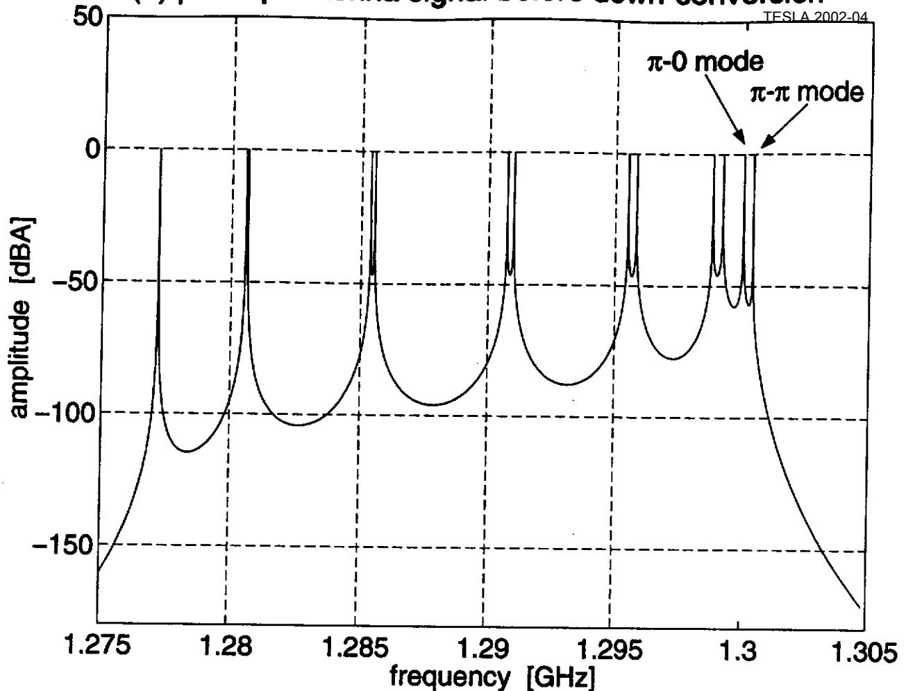
(b) pick-up antenna signal after down-conversion
