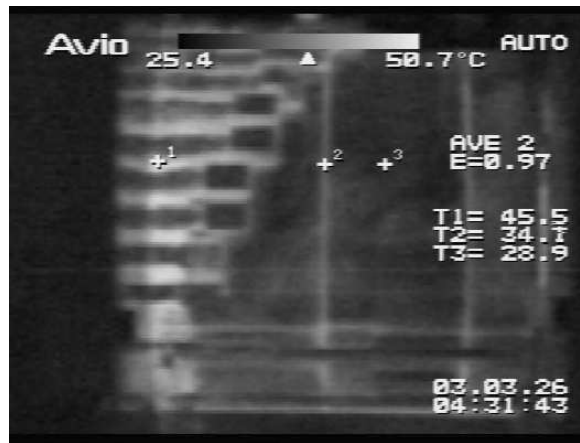
Fig. 6: Infrared camera observation of the RF gun.
