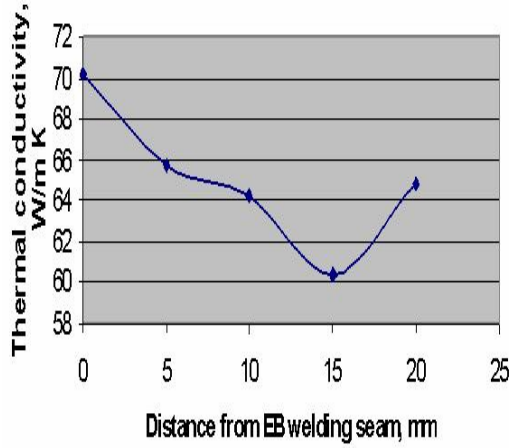
FIGURE 16. Example of thermal conductivity behavior in EB welding area calculated at 4.2K for samples welded at pressure 2.3 \times 10^{-7} mbar.
