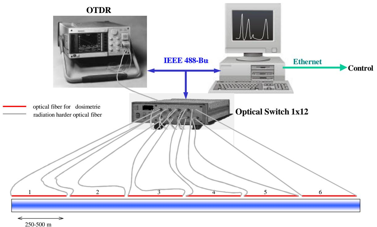
Fig. 6: Measurement set-up for a group of six sensor sections.
