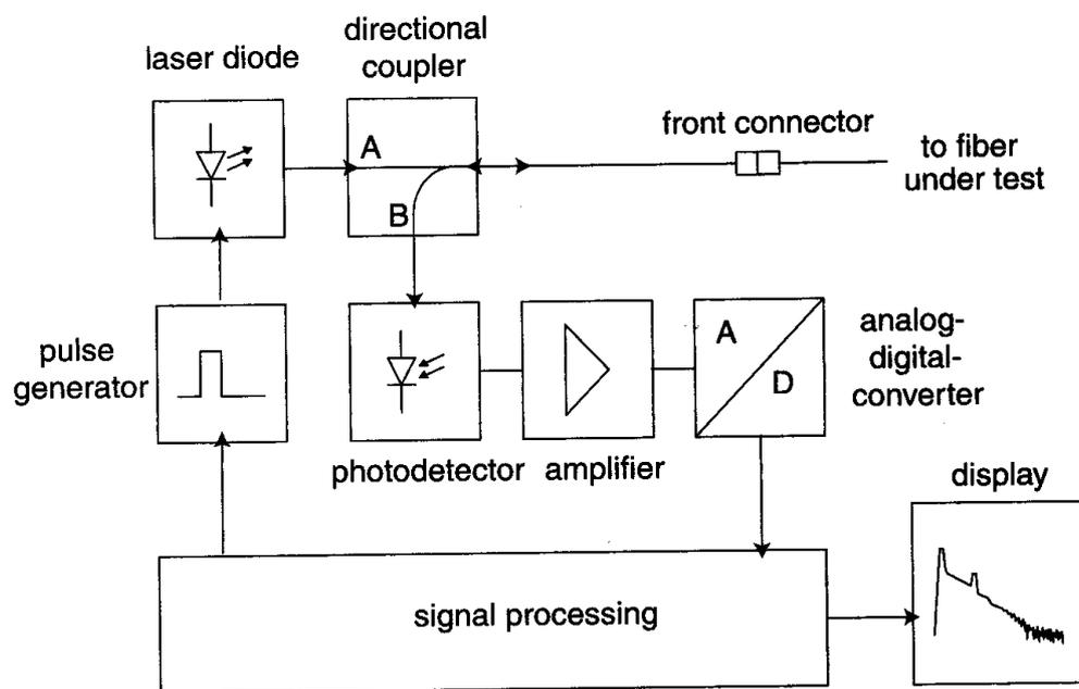
Fig. 1: Block diagram of a single-pulse OTDR.
