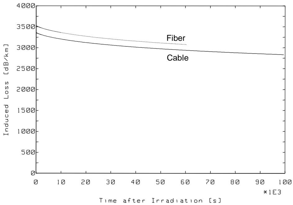
Fig. 3: Increase of attenuation during (above) and its annealing after irradiation (below) of the MM GI fiber FiberCore N1001269E and the cable (diameter 3 mm) made of this fiber. Measuring wavelength 829 nm; <sup>60</sup>Co gamma dose rate 0.047 Gy(SiO<sub>2</sub>)/s; Room temperature.
