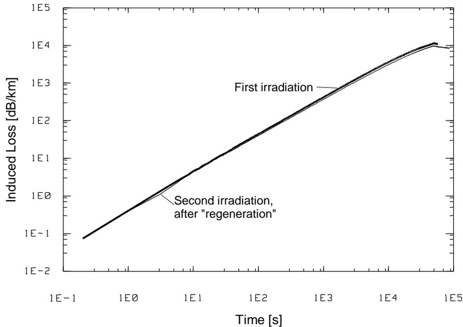
Fig. 5: Behavior of a fiber "regenerated" by heating and high power laser light during a second identical irradiation.
