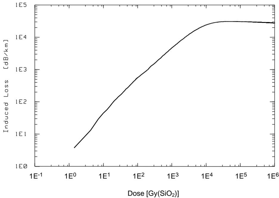
Fig. 4: Loss increase with dose of the fiber FiberCore N2900107GA during  $^{60}\text{Co}$  gamma irradiation with a dose rate of  $1.43 \text{ Gy}(\text{SiO}_2)/\text{s}$ . Measuring wavelength 829 nm, Room temperature.
