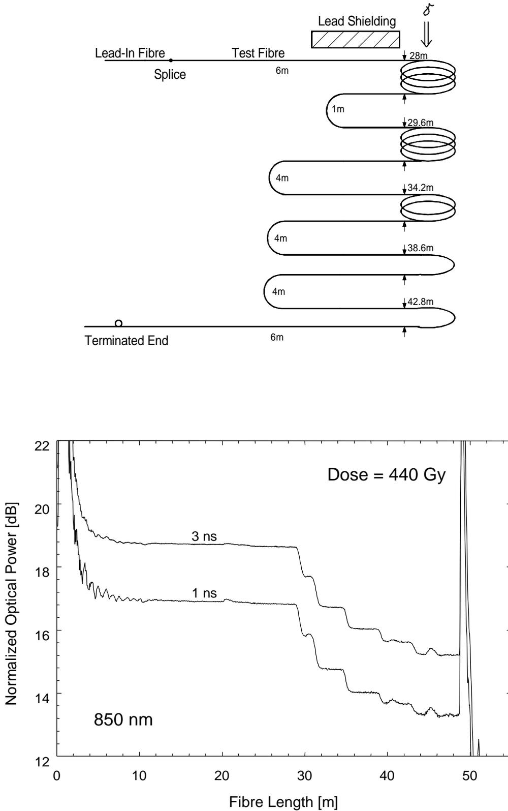
Fig. 2: OTDR traces (below) of the test fiber configuration shown above. The arrows mark beginning and end of fiber spools with three, two and one winding(s), each with a diameter of 6 cm. The measurements were made at 850 nm with OTDR pulse lengths of 1 and 3 ns, respectively, after a dose of about 440 Gy.
