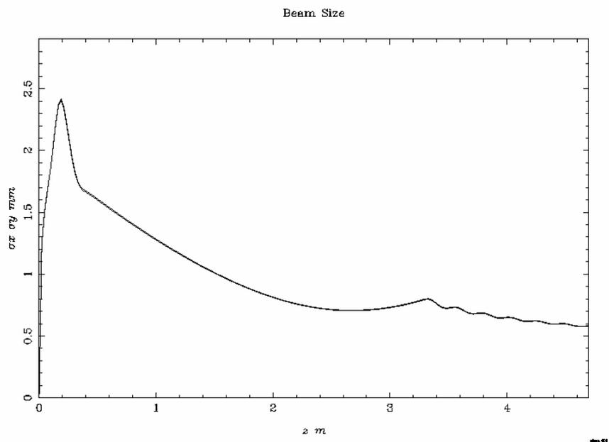
**Fig. 6:** Transverse beam size as a function of position in the 650MHz RF-gun beam line.
