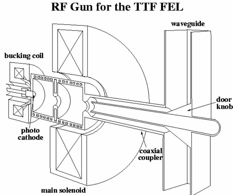
**Fig. 4:** Layout of the TTF-FEL Laser RF-gun.
