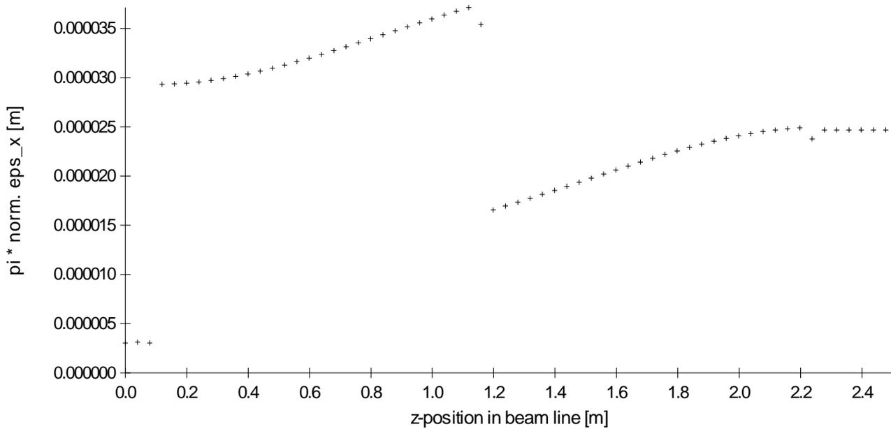
**Fig. 2a:** Evolution of the horizontal beam emittance through the adapter beam line. The solenoid ends at  $z = 0.05$ m.
