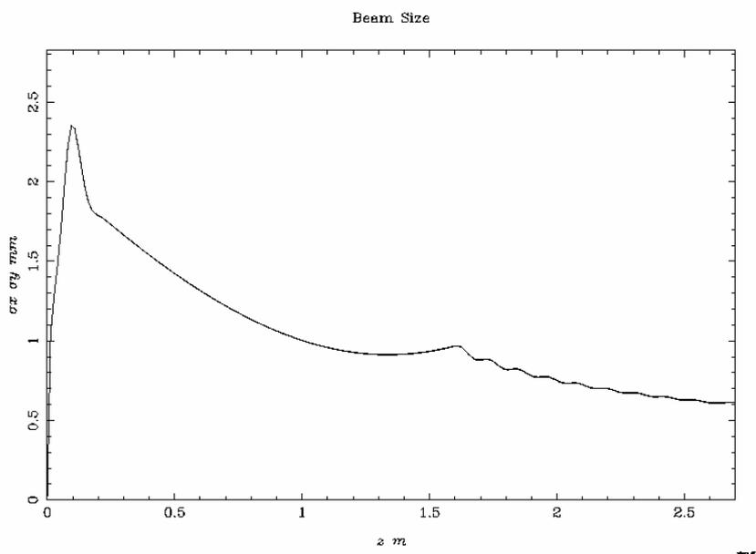
**Fig. 5:** Transverse beam size as a function of position in the L-band RF-gun beam line.
