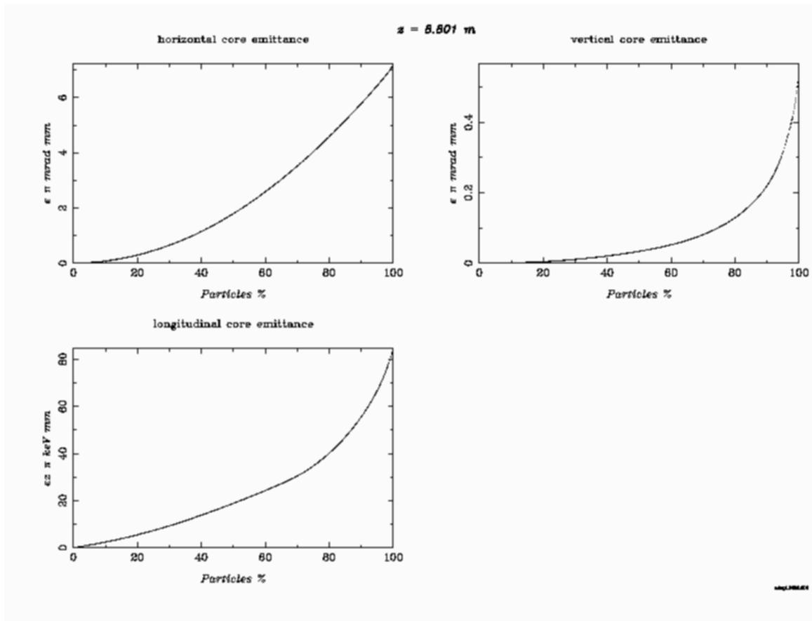
**Fig. 7:** The rms beam emittances (top figures: hor. and vert. planes, lower figure: long. plane) at the end of the 650MHz RF-gun beam line & skew triplet adapter optics as a function of the fractional part of the distribution for  $Q_b = 1.6nC$ .
