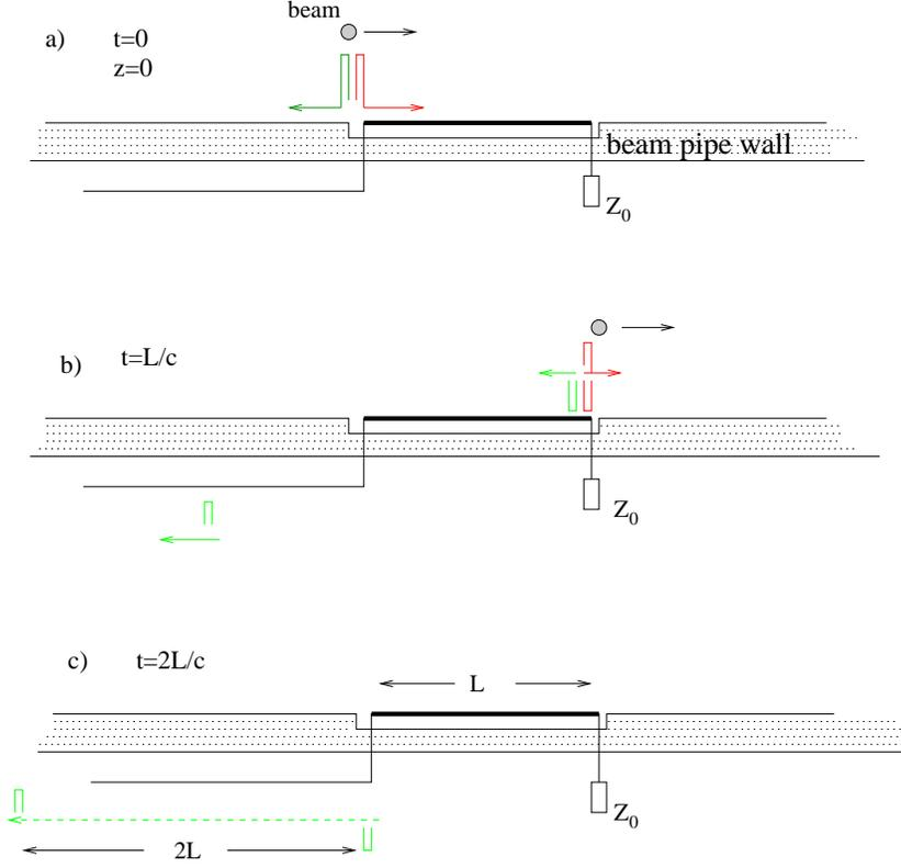
Figure 2: Operation principle of the stripline monitor
