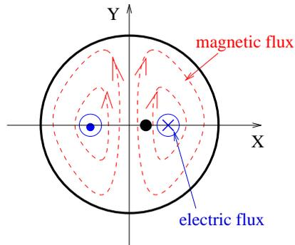
Figure 4:  $TM_{110}$ -dipole mode pattern in the cavity perpendicular to the beam; the black spot indicates the position of the bunch
