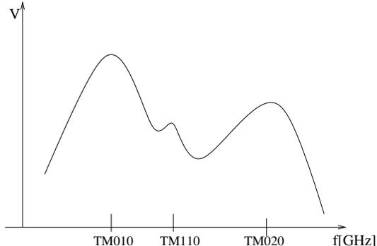
Figure 5: Voltages of the first and second monopole modes together with the  $TM_{110}$  dipole mode
