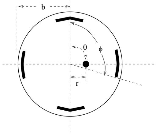
Figure 1: Cross section of the beam pipe with the beam. The thick lines show the cross-section of the stripline electrodes.
