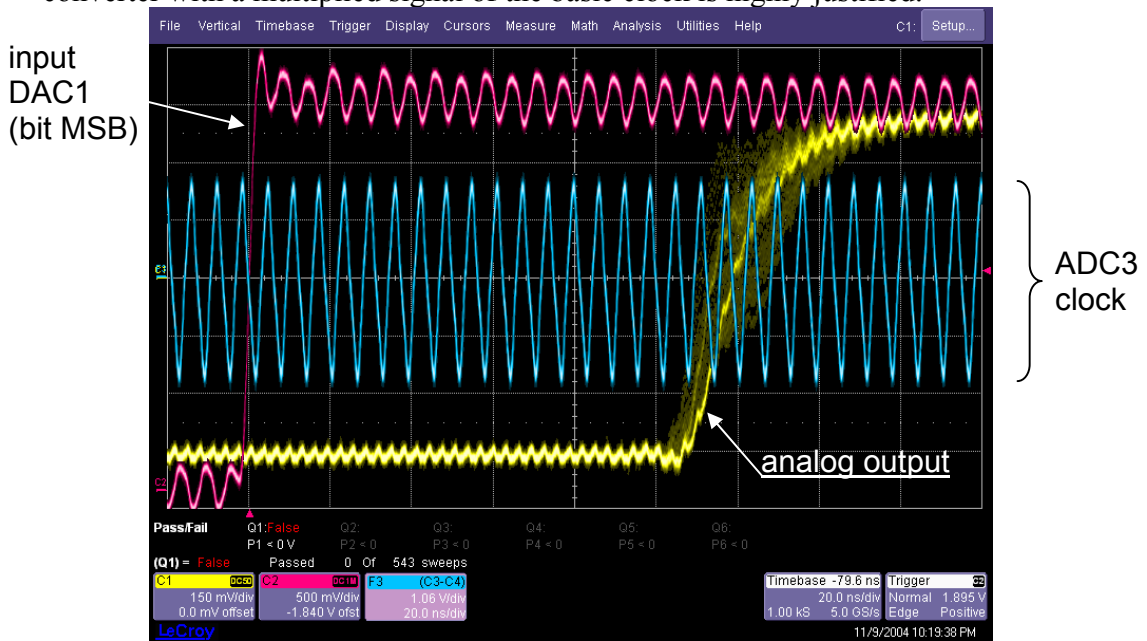
Fig. 16. DAC latency for 160Mpsps.
