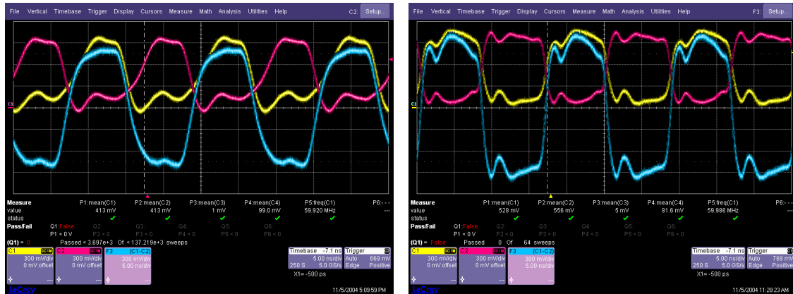
Fig. 11. Differential signal of the 60 MHz clock
