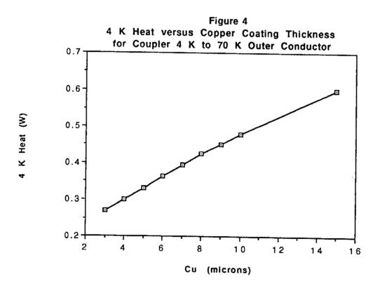
The dimensions for the upper outer conductor in this calculation are: 0.050 cm (0.020 inches) thick stainless steel, 20 cm long, and 10 microns copper plating.
