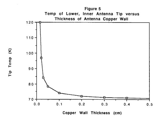
As the thickness of copper decreases below 0.10 cm the temperature of the tip increases rapidly. A solid rod could be used, and has the advantage of no internal vacuum space to pump out, but the disadvantage of a large mass resulting in possible mechanical support and vibration problems. Thermally just copper tube at least 0.10 cm thick is sufficient.
