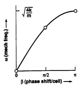
Figure 2b: Dispersion curve for longitudinal vibrational modes.
