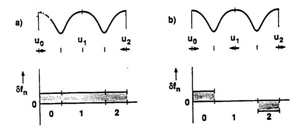
Figure 3a: Displacement u(n) for vibrational  $\pi/2$ -mode and resulting variation in cell frequencies,  $\delta f_c(n)$ .
