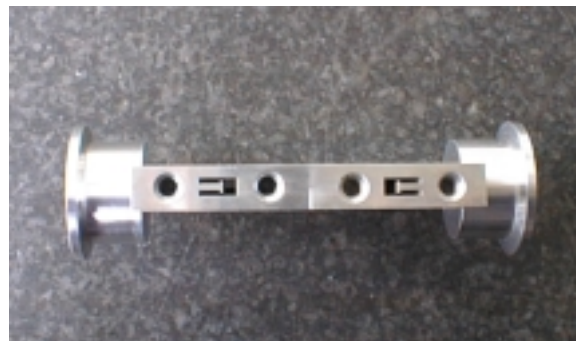
Figure 3 : The prototype chamber profile with the waveguide monitor which will be installed in the third chamber
