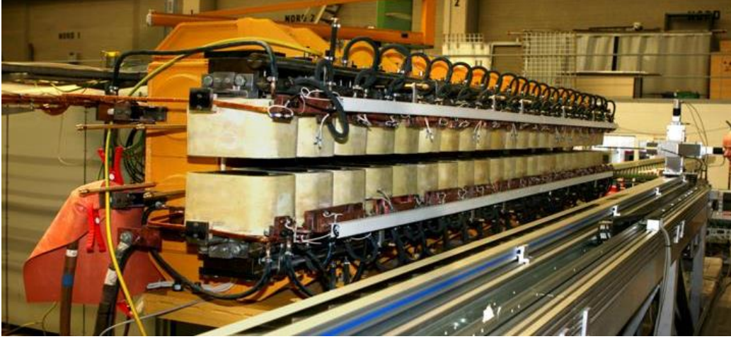
Figure 12: IR undulator at a measurement bench at DESY Hamburg. Previous magnet measurements were done in Dubna and Hamburg for finding optimum settings for correction coils and windings.
