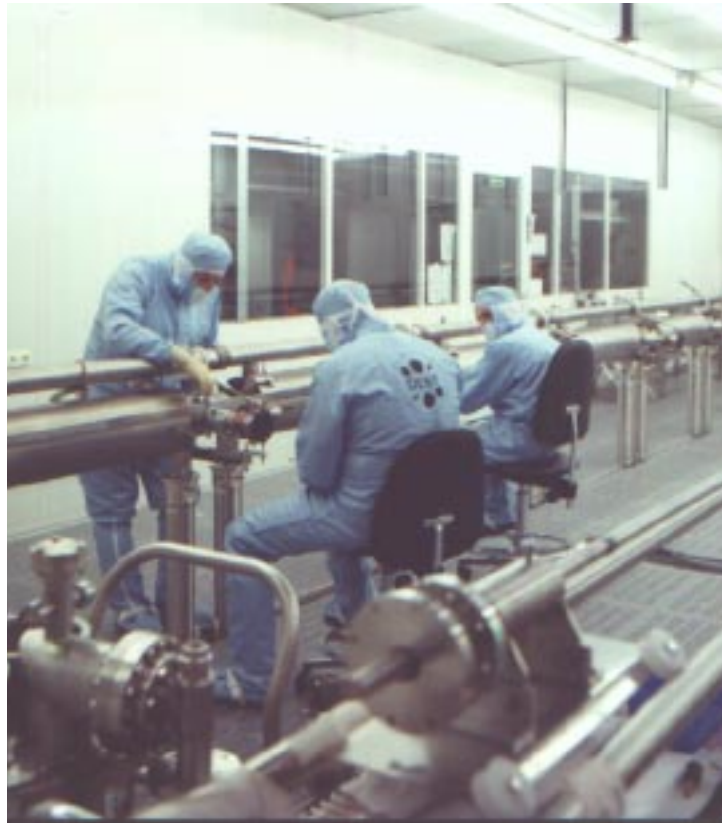
Figure 3.2.3: Assembly of a string of eight 9-cell cavities in the clean room at TTF.
