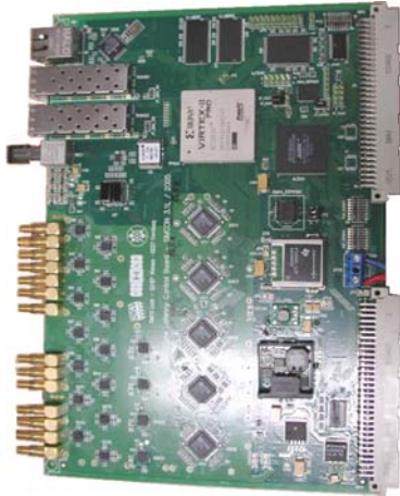
Fig. 2. SIMCON 3.1 controller board
