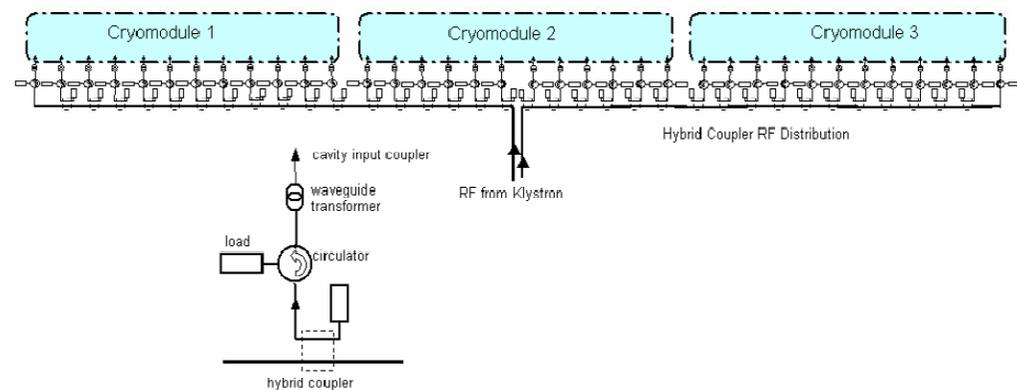
Figure 3.4.5: *RF waveguide distribution of one RF station.*
