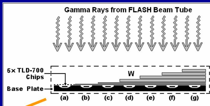
The Lead wedge embedded with TLD Chips
