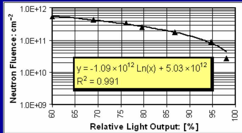
Fast neutron fluence along the FLASH beam pipe estimated with tiny GaAs Dosimeters.
