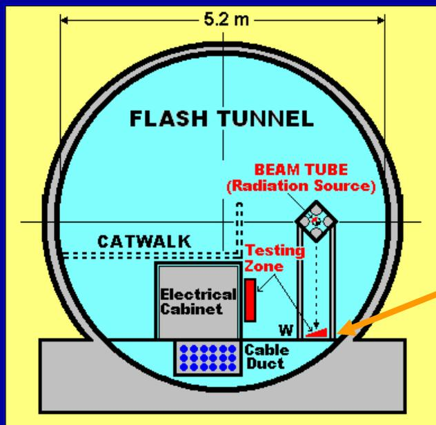
Location of the Lead Wedge in the FLASH Tunnel
