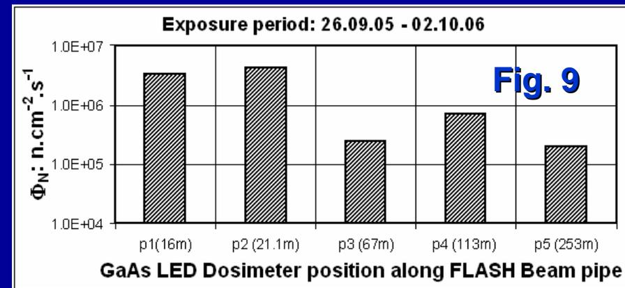
(R5.1) Significant levels of neutron fluence are produced at critical areas (bunch compressors, collimator, injector) due the interaction of “transversally diverted” electrons with the beam tube wall locations p1, p2, p3, p4 and p5 in Fig. 2 )
