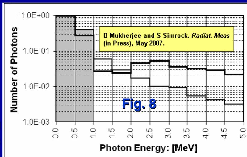
(R4.1) The peak and average bremsstrahlung (BS) photon energy were calculated to be 0.5 and 0.9 MeV respectively
