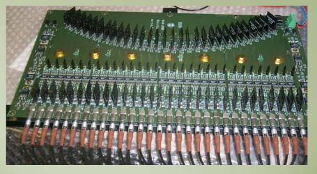
Pyro-electric line detector from individual pyros
