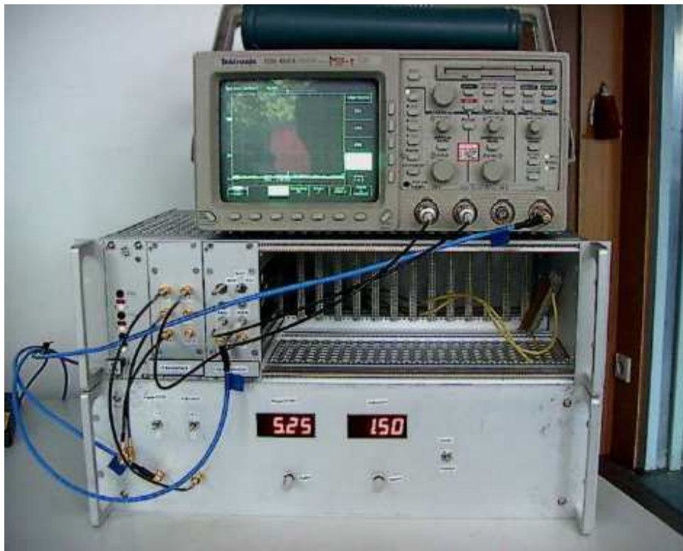
Figure 2.2: Single bunch induced transient detection system version number 1.
