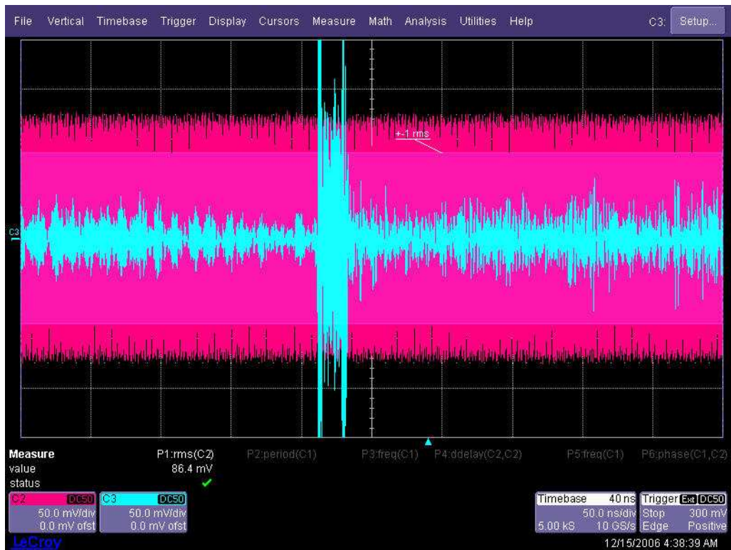
Figure 4.12: 1 nC single bunch induced transient.
