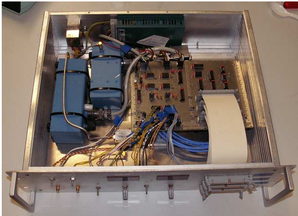
Figure 2.19: Feedforward comb filter version number 2.
