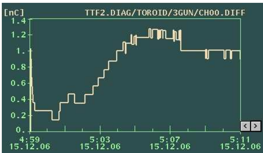
Figure 4.16: Beam charge measured by toroid [nC].
