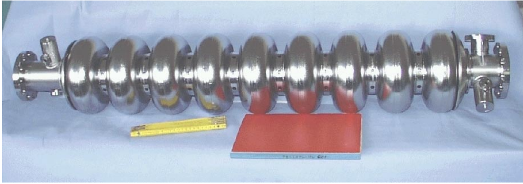
Fig. 4: Photo of the TESLA nine cell cavity with welded HOM couplers.
