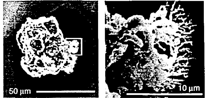
Figures 3a & 3b: A thermal defect (copper)
