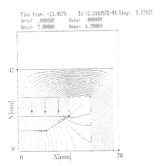
Fig.1: Magnetic field lines over the cross-section of the 0.5 T wiggler.
