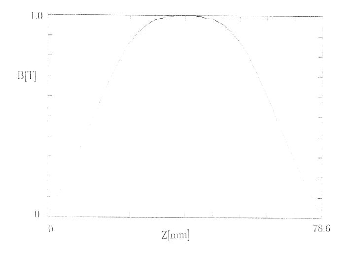
Fig.5: The vertical component of the magnetic field over the half period of the 1 T wiggler.
