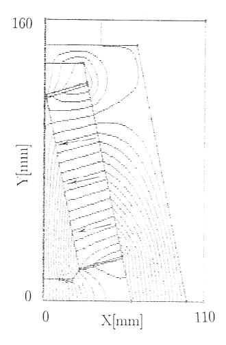
Fig.7: Magnetic field lines over the cross-section of the 1.5 T wiggler.
