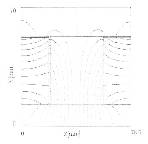
Fig.4: Magnetic field lines over the cross-section of the 1 T wiggler.
