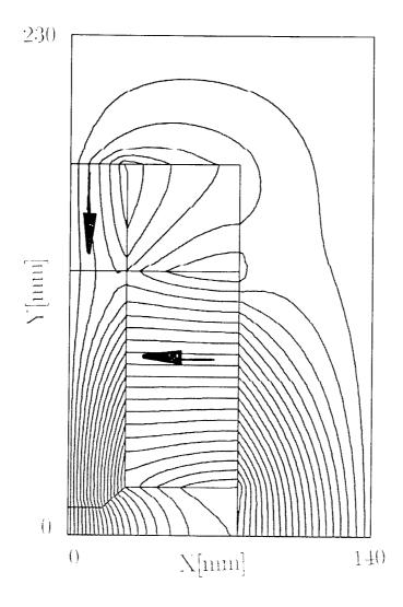
Fig.8: Magnetic field lines over the cross-section of the 2.0 T wiggler.
