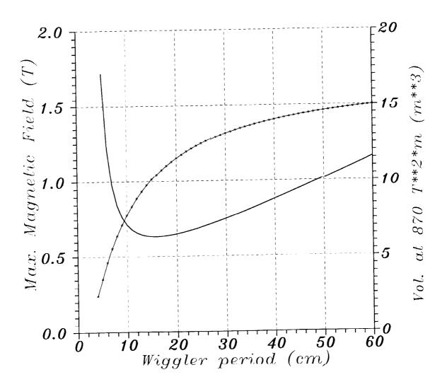
Fig.3: Maximum magnetic field (solid marked line) and required volume of magnetic material (solid line) vs. wiggler period for the Fig.2 design.
