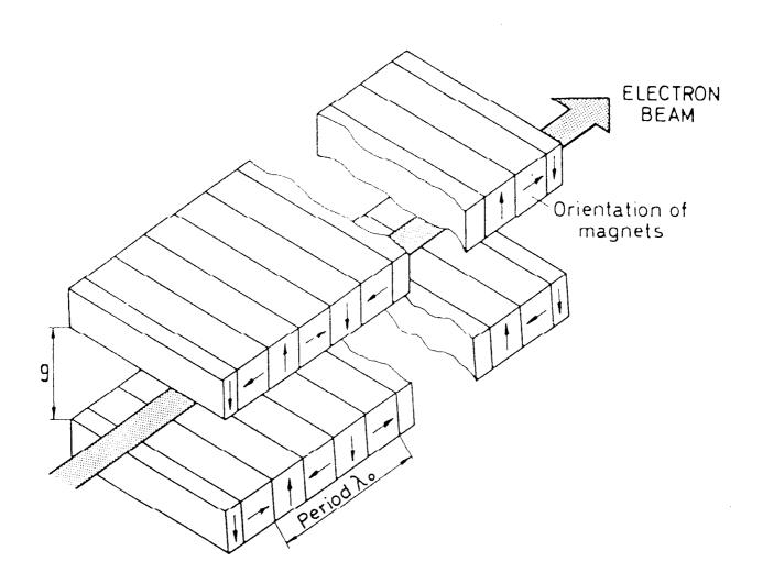
Fig.2: Layout of the 1 T wiggler.
