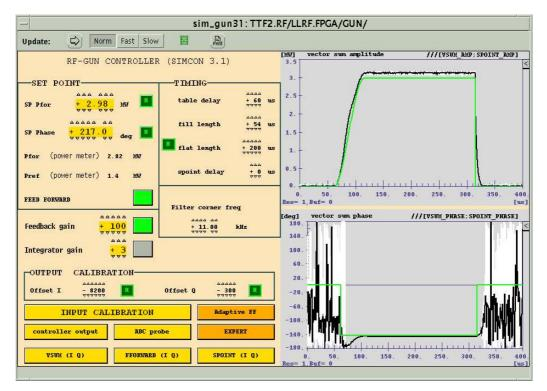
Figure 8. DDD(DOOCS Data Display) panel for RF GUN controller in FLASH. One can see a number of widgets representing various input parameters for control tables generation. Most of these parameters are implemented as callback properties and every user change of theirs values cause the recalculation of new control tables (right site plots).
