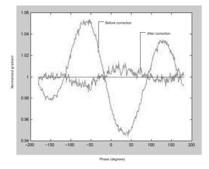
Figure 7. Two plots represent the change of the gradient casued by the change of the set point phase. Before the correction the error was about 12%. After correction it went down to 2%.
