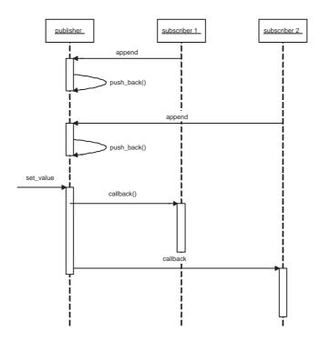
Figure 4. Interaction sequence between publisher and subscriber. Subscriber uses *append* interface to add itself to the subscribers list in the property. When the value inside property is changed, publisher uses *callback* interface provided by subscriber to notify about the change.
