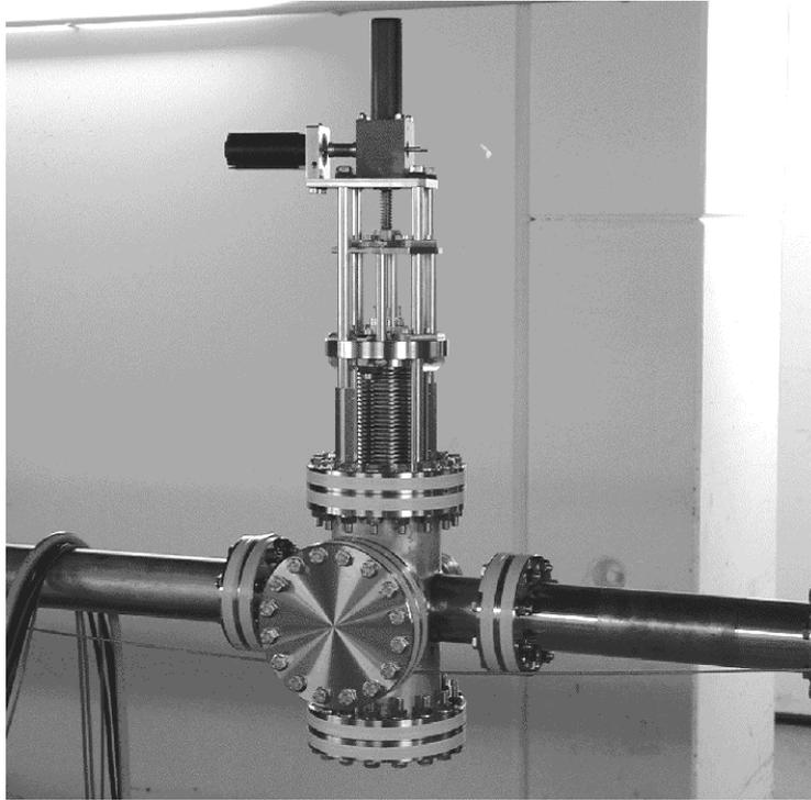
Fig. 5. Photo of radiation detector unit installed at the TTF accelerator
