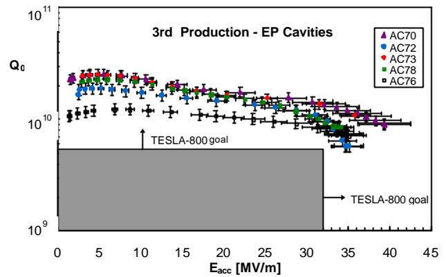
Figure 3: Accelerating gradient vs. unloaded quality factor for several 9 cell cavities from the last production series. These cavities have been electropolished. The results which lie well above 35 MV/m at  $Q_0 > 10^{10}$  surpass the requirement for the 800 GeV version of the TESLA linear collider.
