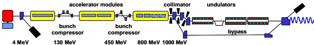
Figure 1: Overview over the VUV FEL. Five cryogenic modules have been installed so far. A sixth module will be installed by 2006. In the remaining space for a possible seventh module presently a transversely deflecting S-band structure has been installed for bunch length measurement.
