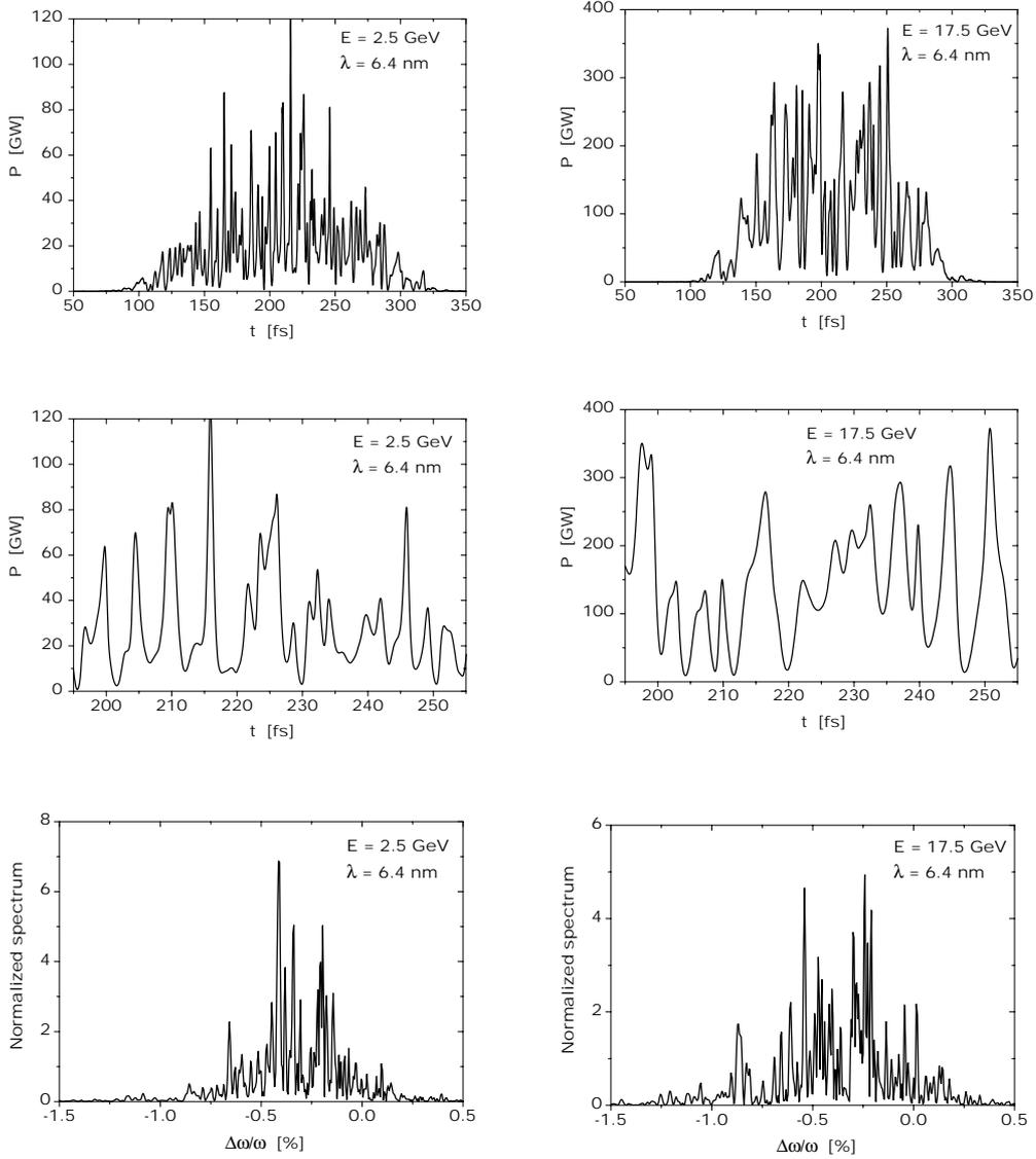
Fig. 10. Temporal and spectral structure of the radiation pulse in saturation regime. Radiation wavelength is 6.4 nm. Left column: low energy option (2.5 GeV). Right column: nominal energy option (17.5 GeV)
