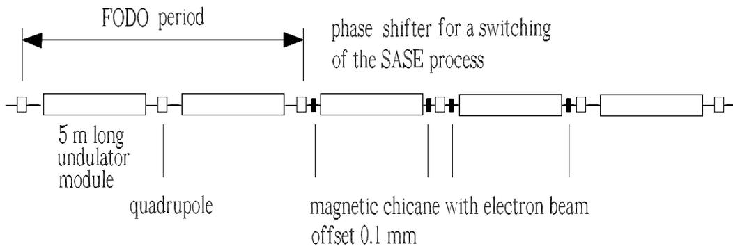
Fig. 7. Installation of an phase shifter in the 3rd SASE undulator
