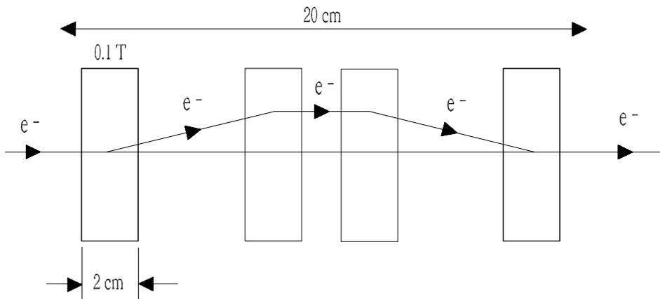
Fig. 5. Electromagnetic phase shifter for a rapid switching of the SASE process in the 0.1 nm undulator
