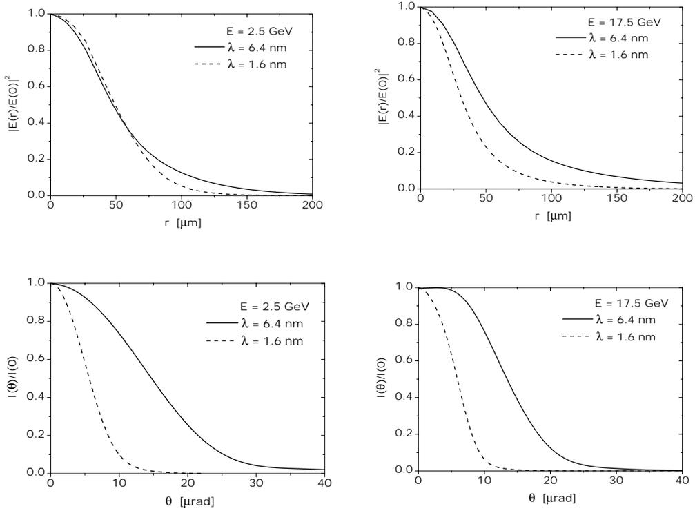
Fig. 9. Intensity distributions of the radiation in the near and far zone in saturation regime. Solid and dashed lines correspond to the radiation wavelength of 6.4 and 1.6 nm, respectively. Left column: low energy option (2.5 GeV). Right column: nominal energy option (17.5 GeV)
