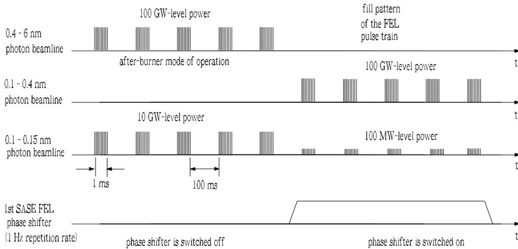
Fig. 4. Photon pulse train patterns for the X-ray SASE FEL
