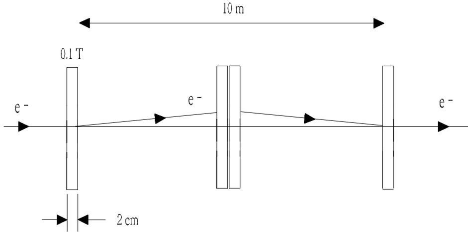
Fig. 6. Electromagnetic phase shifter for a switching of the SASE process in the 3rd (0.4-1.6 nm) undulator
