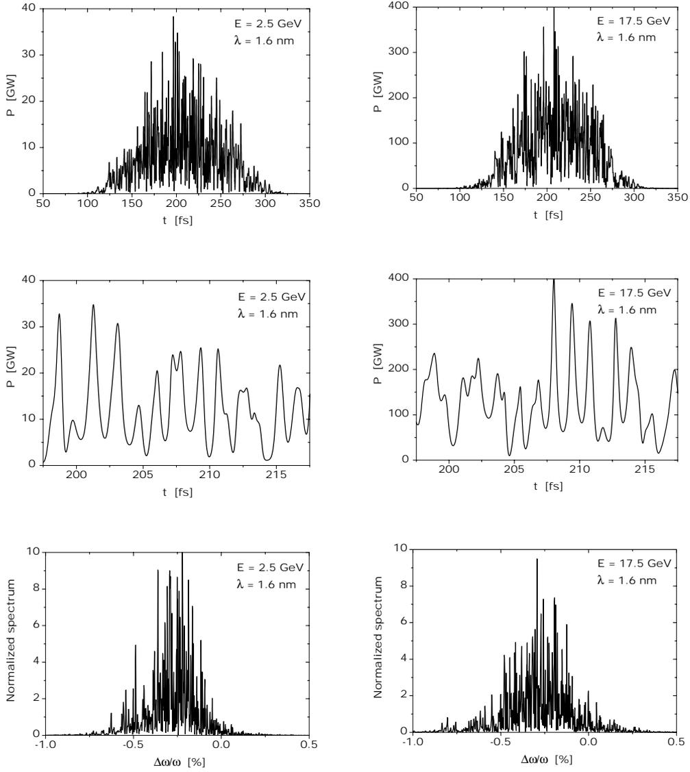
Fig. 11. Temporal and spectral structure of the radiation pulse in saturation regime. Radiation wavelength is 1.6 nm. Left column: low energy option (2.5 GeV). Right column: nominal energy option (17.5 GeV)
