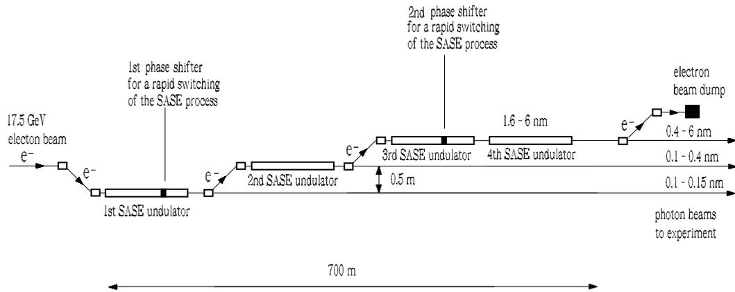
Fig. 2. Schematic layout of the most favorable strategy for VUV radiation. In this scheme it will be possible to provide simultaneously hard X-ray and VUV radiation beams ("after-burner" mode of operation)
