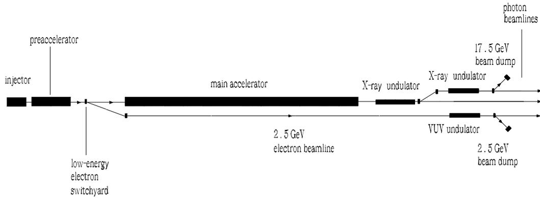
Fig. 1. Schematic layout of the first possible strategy for VUV radiation. This scheme is based on the "electron switchyard" technique
