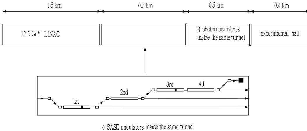
Fig. 3. The schematic layout of XFEL
