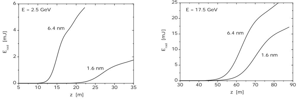
Fig. 8. Energy in the radiation pulse versus undulator length. Left plot: low energy option (2.5 GeV). Right plot: nominal energy option (17.5 GeV)
