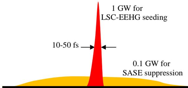
Figure 3: Seed laser profile for LSC-EEHG with SASE background suppression. The central spike is responsible for seeding, while the longer, background pulse is responsible for SASE suppression.
