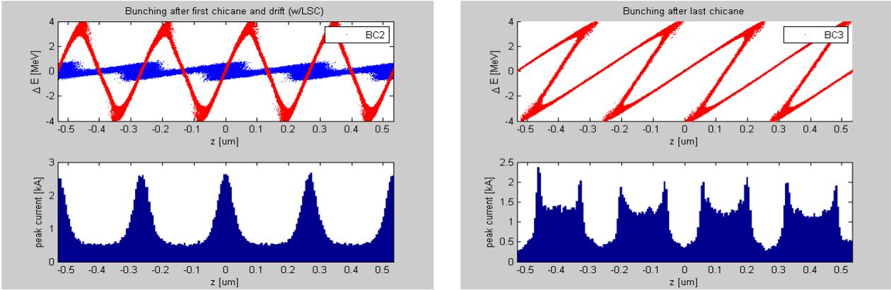
(b.) Initial overfolding (blue) and result of LSC wake (red) on LSC-EEHG seeded portion of bunch
