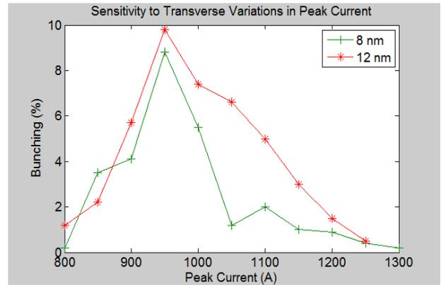
Figure 7: Taking 2% as a lower bound for an acceptable bunching factor, LSC-EEHG at 12 nm in the SASE undulators at FLASH would tolerate transverse variations in the peak current of  $\pm 15\text{-}20\%$ , providing seeded bunching for a majority of the charge in the bunch. For shorter wavelengths, the tolerance is tighter.
