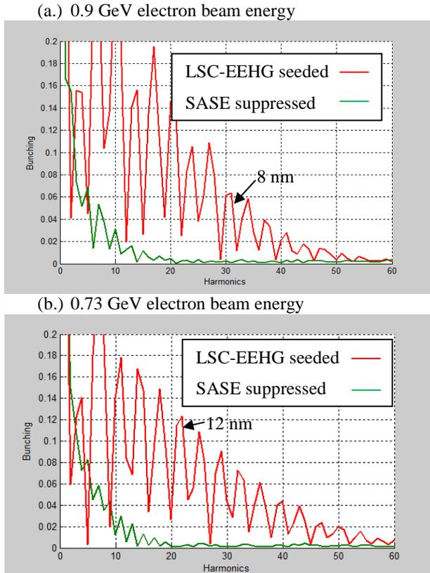
Figure 4: Harmonic content after last chicane for seeded and suppressed portions of the beam at different electron beam energies. Seeding was done with 266 nm in both the background and in the central spike.
