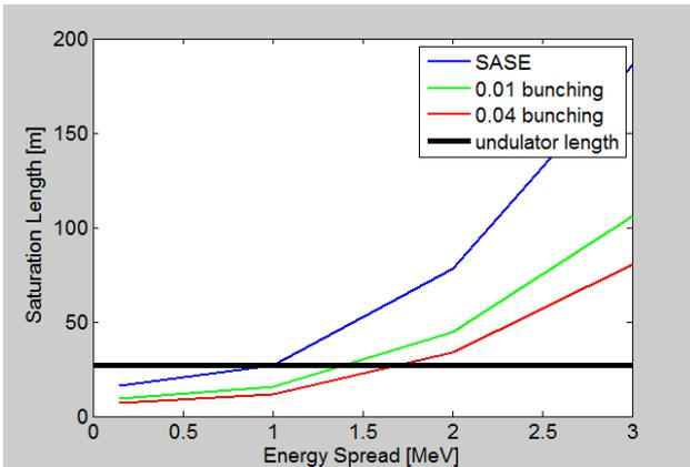
Figure 8: Saturation length as a function of rms slice energy spread for different initial bunching factors generated by the Xie 3D model [7] and Eq. 4 [8]. A 1 kA peak current was used at a beam energy of 0.73 GeV.
