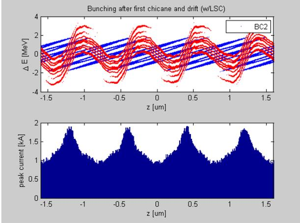
(b.) Bunching pattern of seeded portion of beam prior to radiator
