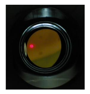
Figure 9: View through the diamond window onto the transition radiation screen. The red spot is light from an alignment laser. The window was fabricated by Diamond Materials GmbH, Freiburg.
