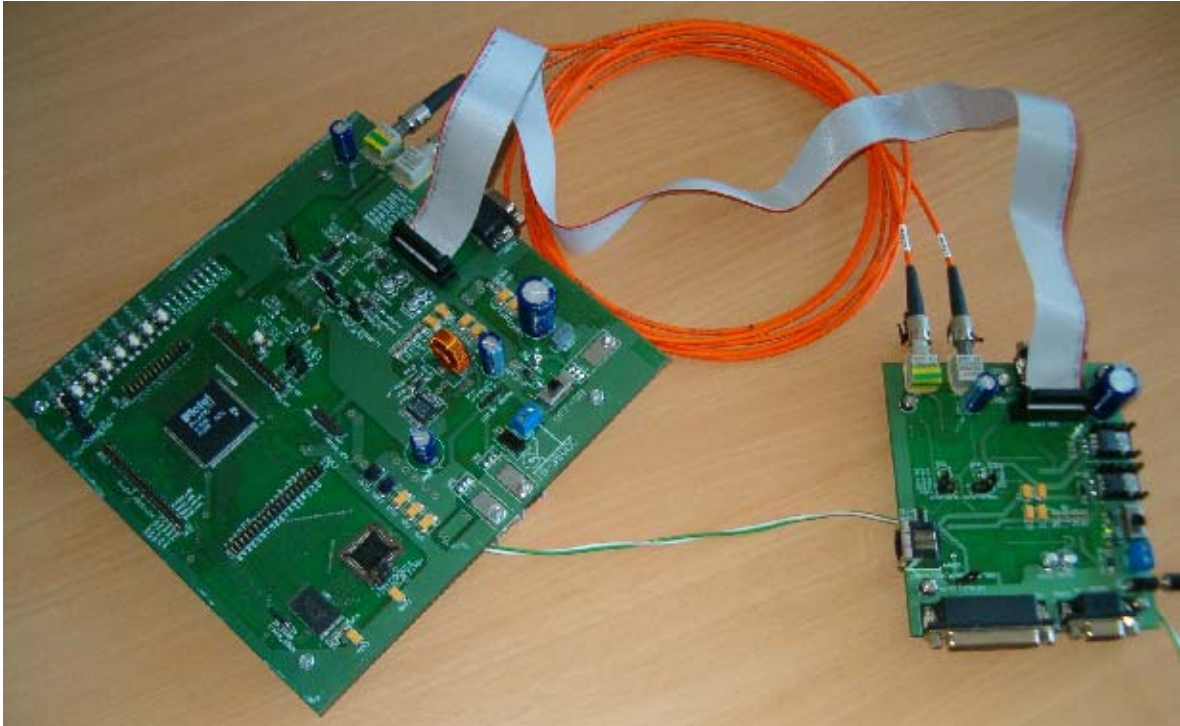
Figure 6.13. The FPGA and transceiver boards interconnected with full-duplex fibre optic link and 20-wire ribbon cable
