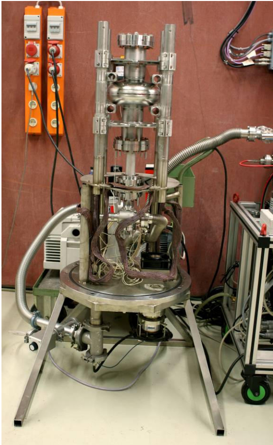
Figure 16: Baking installation at DESY.
