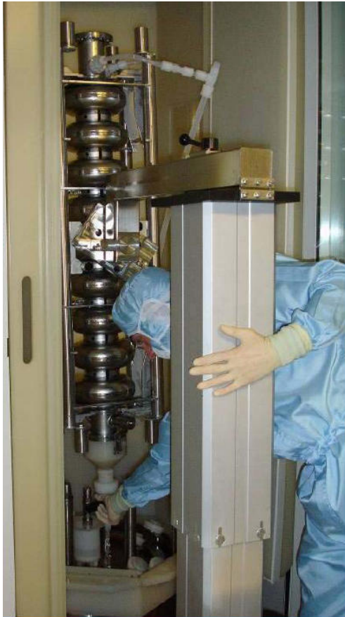
Figure 11 DESY HPR Set-up
