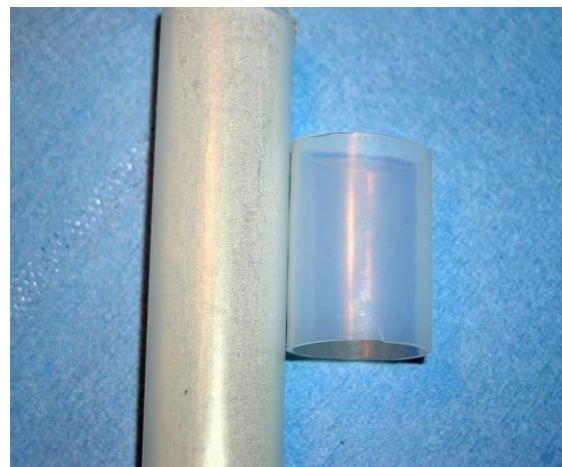
Figure 5: Tube before and after ethanol rinsing
