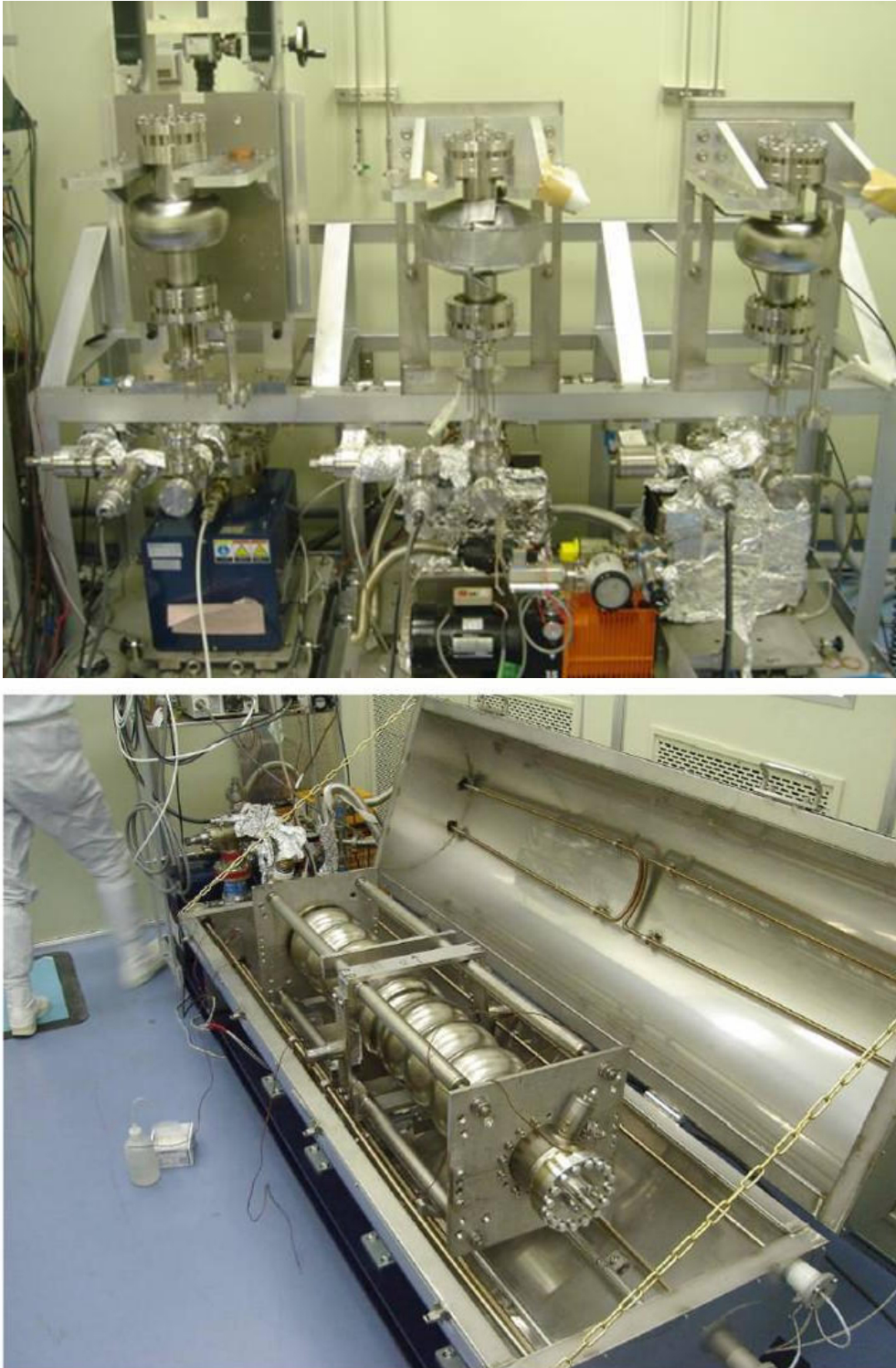
Figure14: Baking installation at KEK for single and multi-cell cavities.
