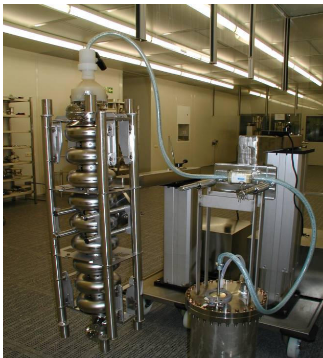
Figure 6: Set up of alcohol cleaning apparatus at DESY
