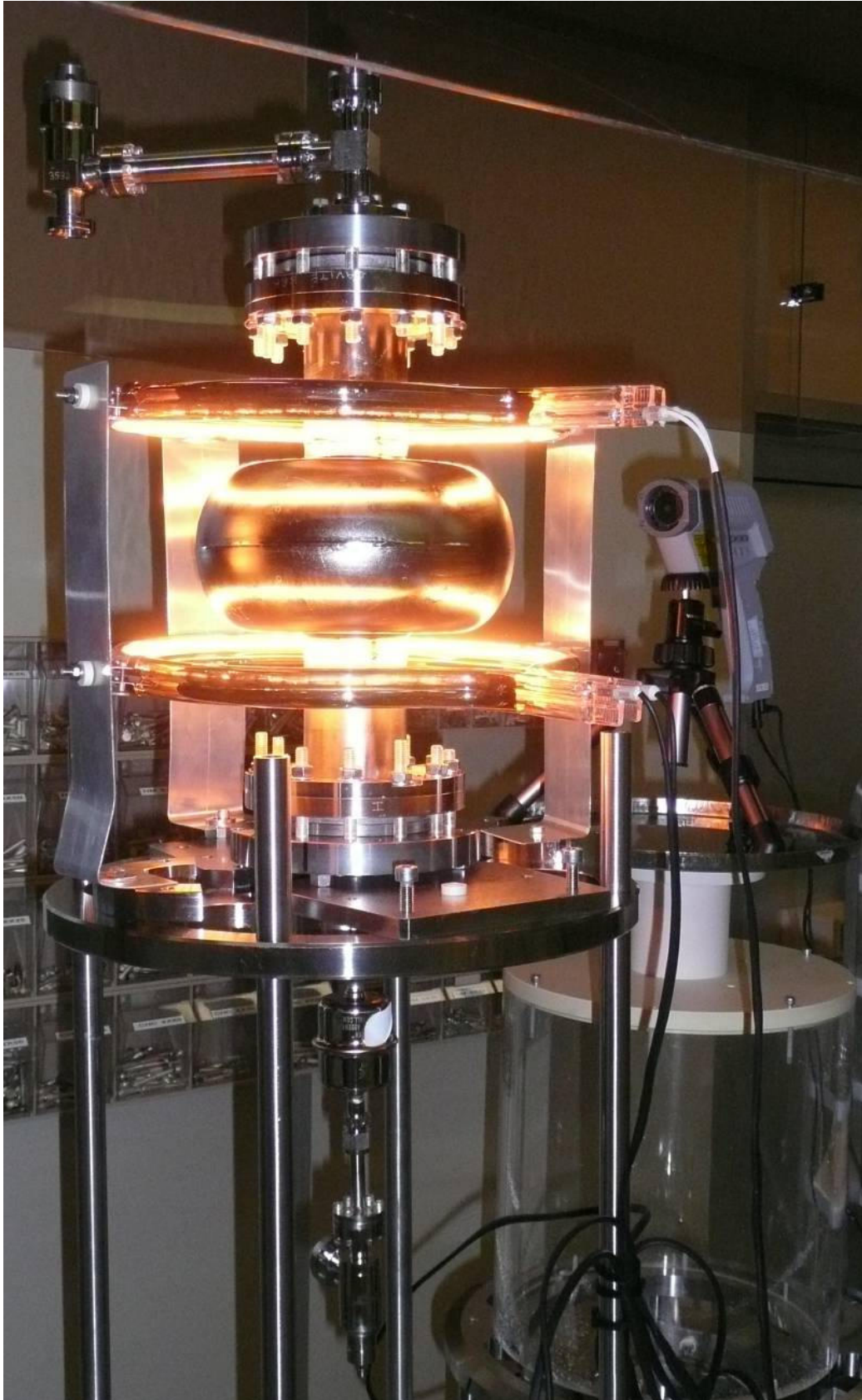
Figure18: "Fast Baking" at Saclay with infrared heaters.
